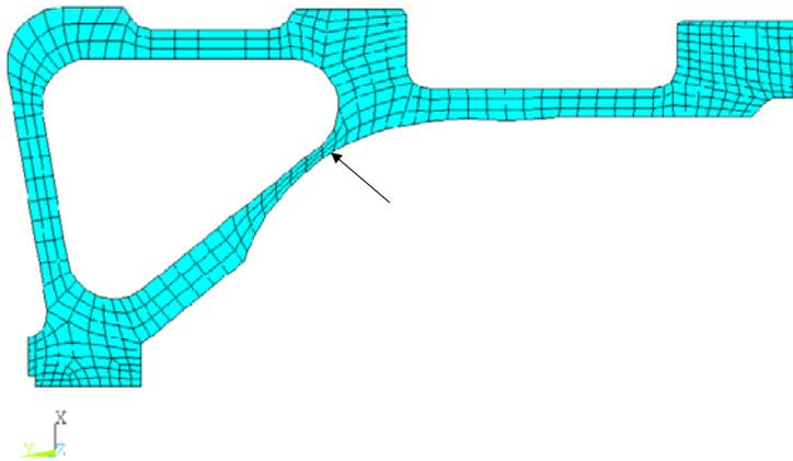
Figure 2 Perturbed Mesh After Moving the Controlling Node
